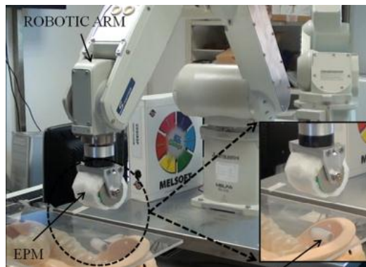
Robotic arm moving the permanent magnet (EPM) used for capsule navigation and tissue scraping
